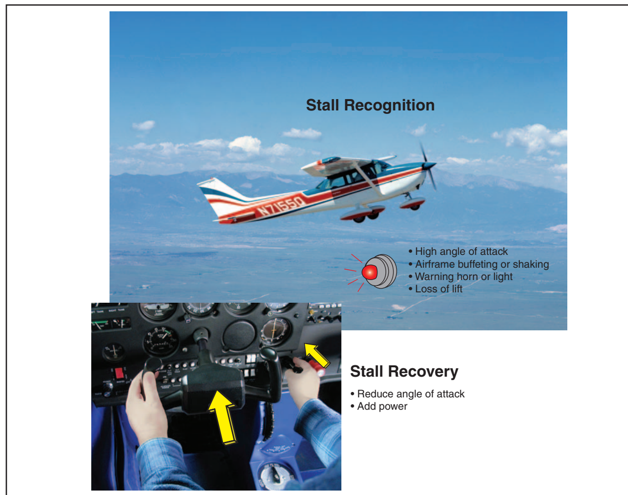
Figure 4-3. Stall recognition and recovery.
